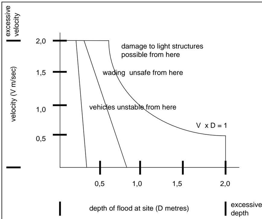
**Figure 9:** The relationship between velocity and depth of flooding with a certain level of hazard as a result
