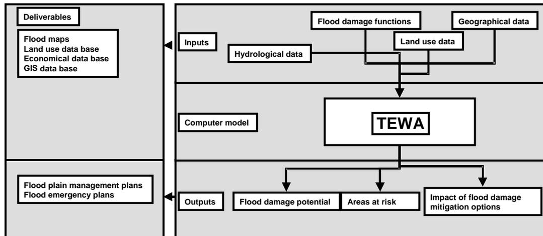
**Figure 3** The process of calculating flood damage by using TEWA
