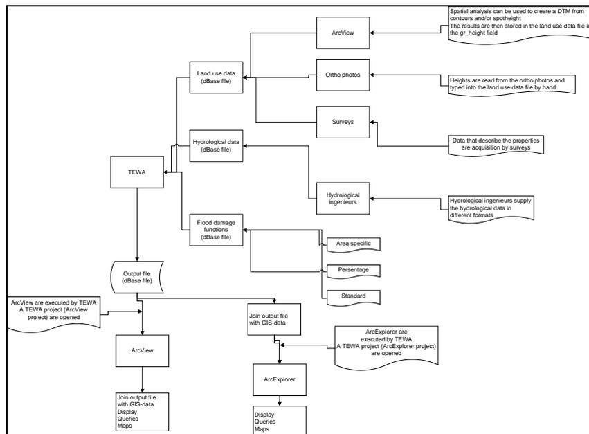
**Figure 4** The methodology of TEWA to calculate flood damage
